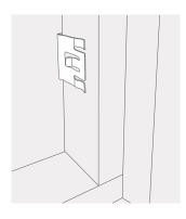
TIP: A credit/debit card can be used as a template to align the top & bottom holes. Place the card as shown.
